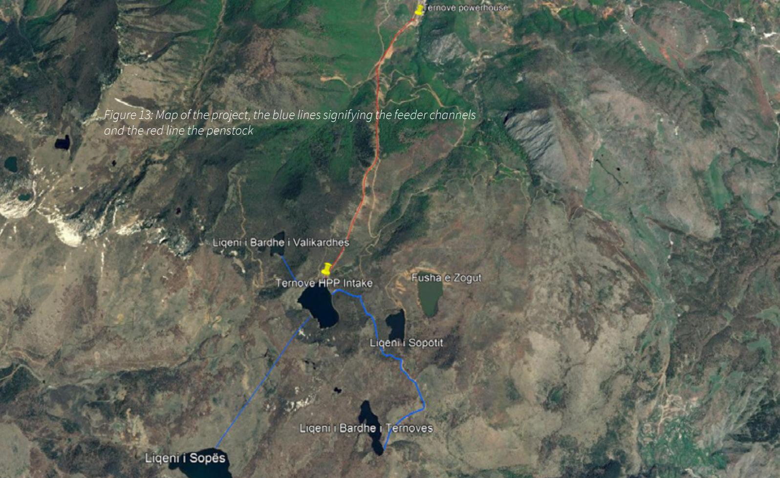
Figure 13: Map of the project, the blue lines signifying the feeder channels and the red line the penstock
